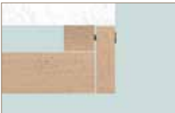
covering the hollow chamber with end plate
