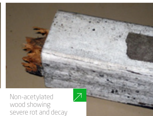
Non-acetylated wood showing rot and decay
