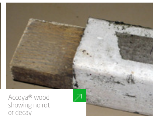
Non-acetylated wood showing severe rot and decay
