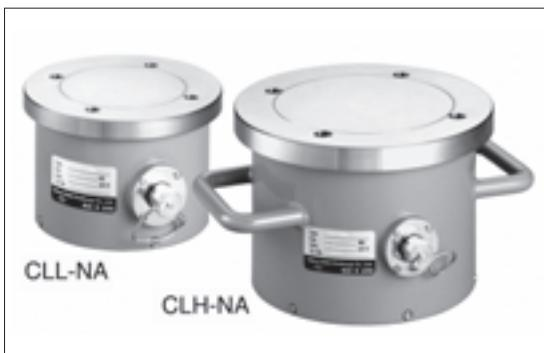
The CLL-NA and CLH-NA load cells with a flat loading platform are used to conduct loading tests on cylindrical concrete specimens. A cylindrical concrete specimen can be directly set on the surface of the loading platform. Guide markings are shown on the loading platform so that each specimen different in size can be placed in alignment with each appropriate guide marking.
