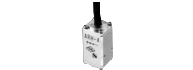
The ARH-A acceleration transducer has a waterproof structure. It is installed in water or ground or embedded in concrete. The rigid waterproof structure makes this transducer suitable for use in an adverse environment or for outdoor use.
