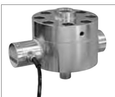
The TLJ-NA Tension Load Cell is designed considering JIS B 7728 "Load calibration devices for verifying material testing machine" and is the most suitable for verification of single axis tension testing machine. Calibration in accordance with JIS B 7728 is available at extra cost.
