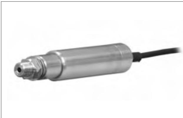
The PWA pressure transducer is a strain gauge pressure transducer with built-in amplifier. As the model equipped with a fluoroplastic input/output cable, a high temperature pressure measurement is available up to 120°C. This model consists of two types of outputs for voltage and current and five ranges of 2, 5, 10, 20 and 50MPa.
