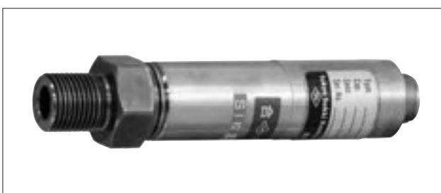
The PWH-PA high-capacity pressure transducer has a sealed structure made with high-strength stainless steel. Using this highly sensitive transducer, stable high-accuracy measurement can be made over a long period of time. It is used to control plant or production lines, to measure jack pressure, and for various other applications.
