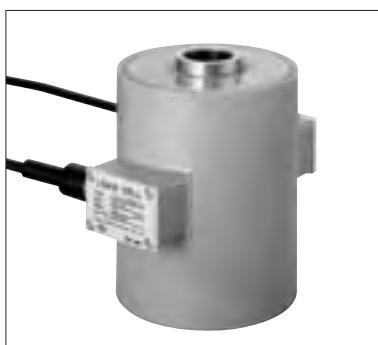
The TCLU-NA-D Tension/Compression Universal Load Cell is a TCLU-NA load cell with two isolated I/O ports. One Input/Output cable can be connected to an analog measuring instrument and the other to a digital measuring instrument at the same time with no chance of interference between the two instruments.
