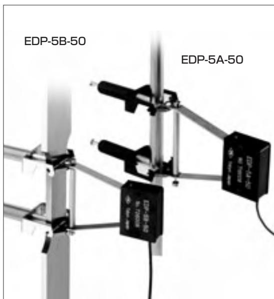
The EDP series Displacement Transducer is designed to measure elongation in round metal rod and sheet metal test specimen. It has a special holder that simply and securely holds it in place, and it detects elongation in test specimen based on displacement between two knife edges. This series uses a strain gauge for the sensing element and can be connected to an ordinary strainmeter for high precision measurements.
