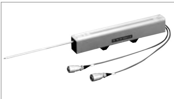
The SDP-D-D displacement transducer is the SDP-D displacement transducer with dual isolated I/O ports. For example, one set of input and output cables can be connected to an analog measuring instrument and the other set to a digital measuring instrument. With two different types of measuring equipment connected to this transducer, simultaneous measurements can be made without interference.
