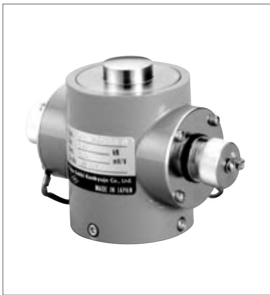
The CLP-NB-D Load Cell is a CLP-NB type load cell with two isolated I/O ports. One Input/Output cable can be connected to an analog measuring instrument and the other to a digital measuring instrument at the same time with no chance of interference between the two instruments.
