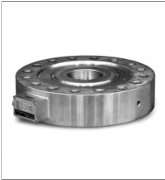
The TCLY-NA is a Tension/Compression Universal Load Cell with low-profile construction and high-capacity. It offers high precision, high output characteristics and an excellent stability because it uses a shear beam for the strain sensing element. This model is widely used in applications like one-axis loading test machine.
