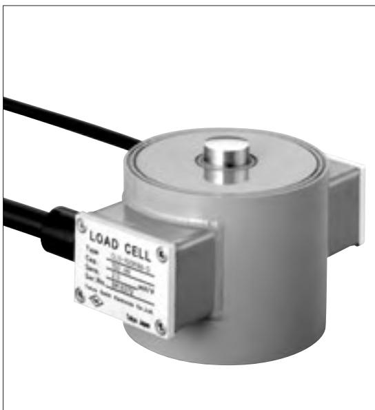
The CLU-NA-D Load Cell is a CLU-NA type load cell with two isolated I/O ports. One Input/Output cable can be connected to an analog measuring instrument and the other to a digital measuring instrument at the same time with no chance of interference between the two instruments.
