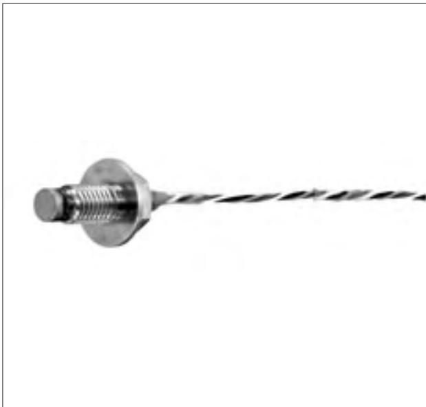
The PWFD-PA is a bolt-shaped flush diaphragm pressure transducer. As it is small and can be used for dynamic measurement in high temperature region, it suits various pressure measurements around engine. The shape of hexagonal bolt with flange makes installation to a screw hole easy.
