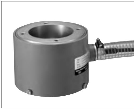
The KCE-NA Load Cell is a center-hole-type load cell designed to use in tension measurement of anchoring strand. It can deliver stable measurement performance under somewhat eccentric load. An extra model with built-in temperature sensor is available.
