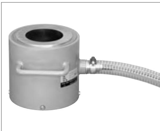
The KCM-NA Load Cell is a center-hole-type load cell with a strain gauge mounted on a cylindrical strain sensing element. It is used to measure prestress or tension force on ground anchors, pullout testing and measuring axial force on tie rods. The model is especially well suited for measuring on site.
