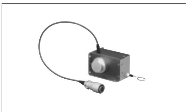
The DP-E displacement transducer is used to measure a large amount of displacement. A stainless steel wire is drawn to measure displacement. The wire tension is constant in the same direction regardless of the amount of displacement. This is a small, lightweight, and high-accuracy transducer.
