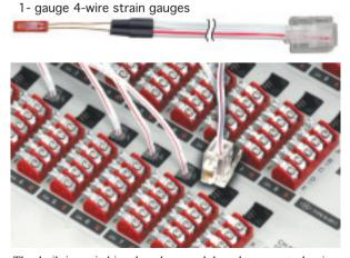
The built-in switching box has modular plug receptacles in addition to conventional terminal boards and NDIS connectors.
