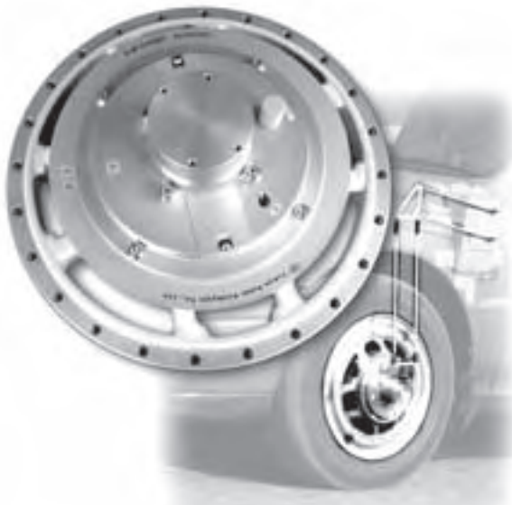
Rotary encoder type angle detector onboard model imaged
