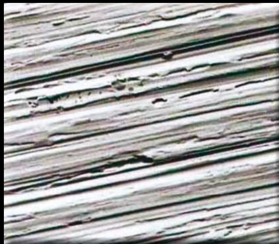
Ground with grain 320, magnified 650 fold
