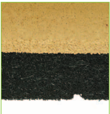
The cross-section through the tile shows the dual-layer construction with the through coloured EPDM layer.
