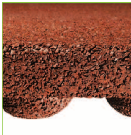
The cross section shows the homogeneous granular structure.
