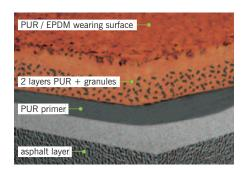
This is a high performance surface with a relatively low level of force reduction. The homogeneous and seamless wearing surface is identical to the topping of the Regupol AG system. The entire system conists of three polyliquid layers
