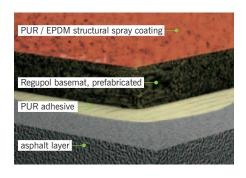
Waterpermeable or impermeable surface for athletic tracks and multipurpose facilities. The wearing surface is a structural spray coating consisting of a special PUR compound premixed with selected EPDM rubber granules.
