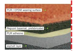
The traditional system for international competition. The wearing surface consists of an impermeable PUR coating with selected EPDM granules broadcast into the 'freshly' applied PUR compound resulting in a homgeneous and seamless granulated topping. The basemat
