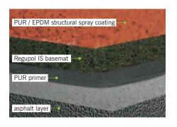
Generally, the Regupol PD-IS is installed as a permeable system on top of a permeable substructure. The wearing surface is the same than that for the Regupol PD system. It is also a more economical solution and due to its slightly rough surface texture it is a perfect fit for athletic tracks and/or multipurpose courts.
