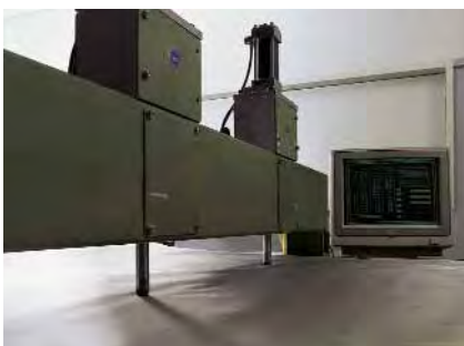
Thickness Control of Woven Wire Cloth
