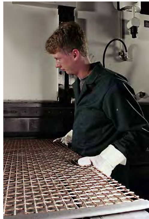
Production of hook strips
