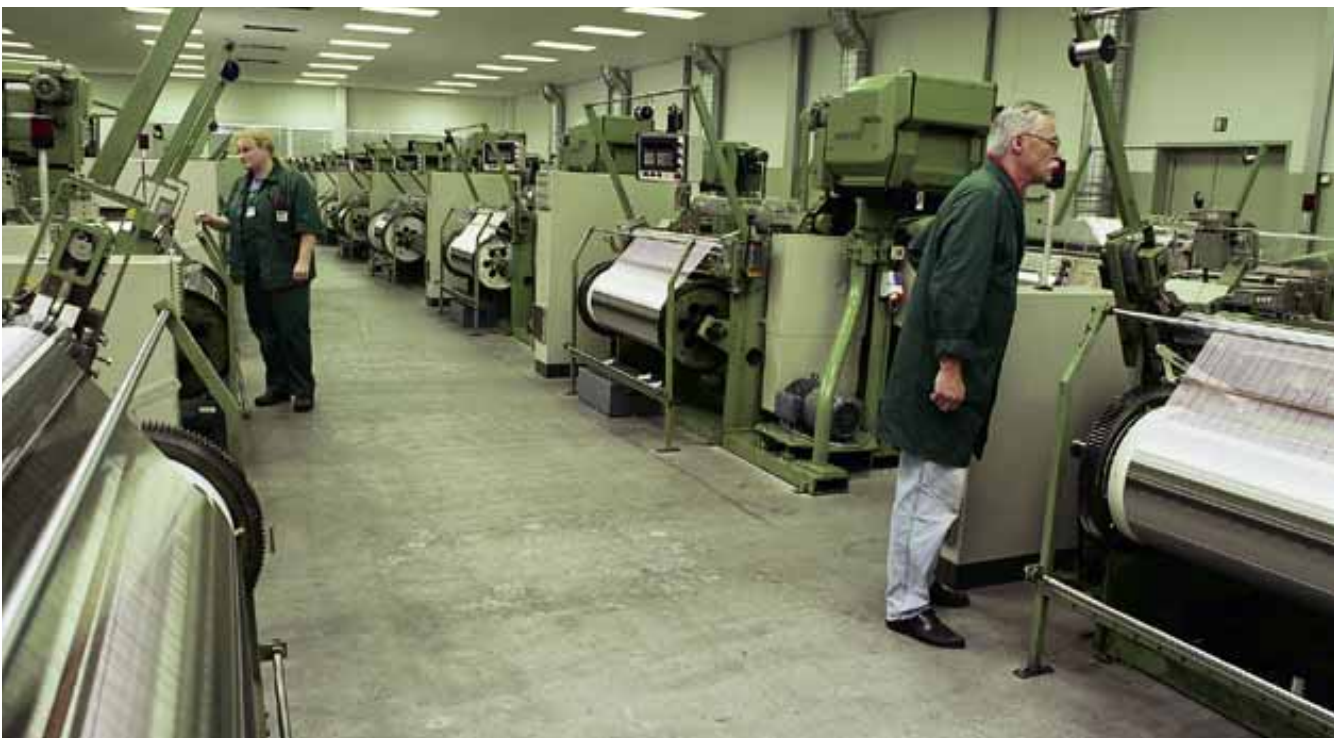
Production of fine mesh woven wire cloth
