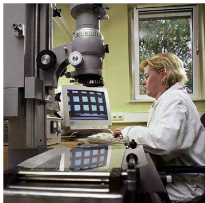
Mesh aperture measuring in our laboratory
