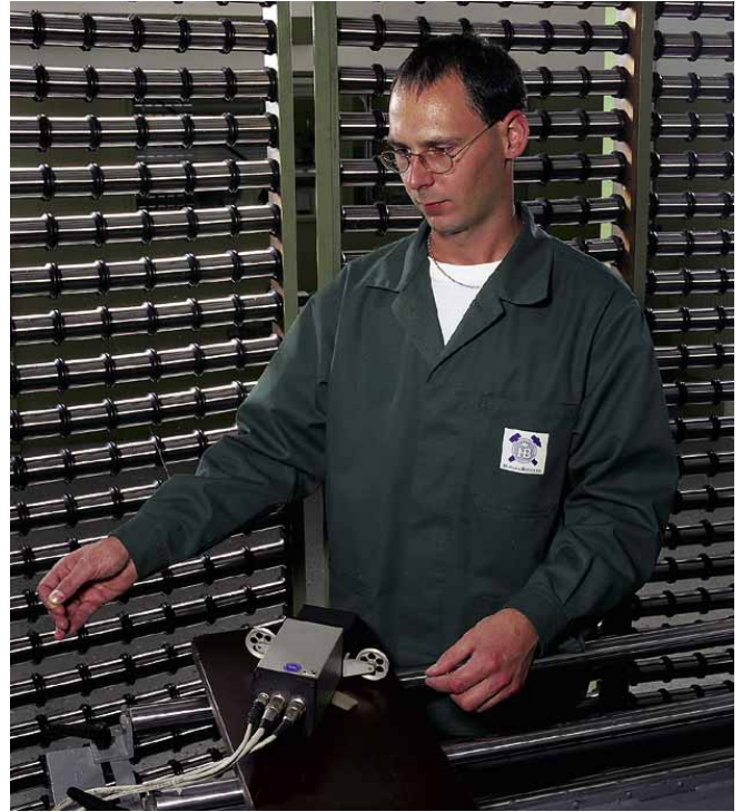
Quality control of warp wires
