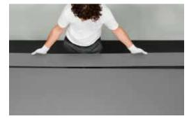
For cuts on the long side of Laminam 1000x3000 mm, position the slab on a stable and flat plane and fasten a standard aluminum rod on the surface to be etched. Cut and shear as described in figures 17, 18, 19. Take the slab with open arms on the long side and, starting from the already opened edges, slightly press downwards till shearing completely.
