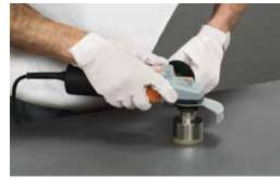
For holes with diameter over **8-10 mm**, use diamond cup cutters mounted on drills or on grinder. Start drilling keeping the tool sloped to the slab. These tools can be used dry or with water.
