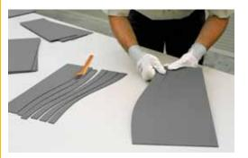
Slightly bent cuts can be obtained using a manual glass cutter. They can be more bent by using Laminam 3 slabs.
