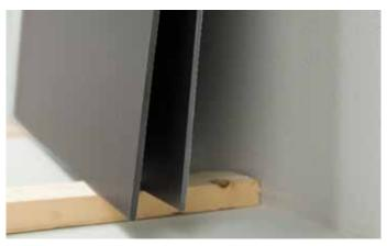
Lay the slab gently on the long side, keeping it slightly sloped and caring to arrange it on soft material or suitably spaced wooden strips.
