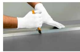
Etch the slab surface from the edge outside to edge outside, without never detaching the blade from the etching axis and keeping it perpendicular to the surface. Do not interrupt nor restart cutting and press steadily and evenly.
