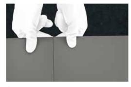
Chop off the etched surface at the edges to aid the cut fracturing. For dimensions larger than 1000 mm open the cut by shearing from both etched edges.
