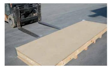
To lift and move crates of slabs **1000x3000 mm**, using fork lifts or yard cranes, it is important to get the package in the long side, caring to position in its center, extending the forks as much as possible as they have to grip all through the pallet depth.
