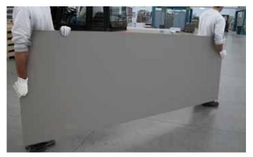
Handle the slab with the aid of a second operator, keeping it always perpendicular to the ground, without bending and protecting corners against accidental impacts.
