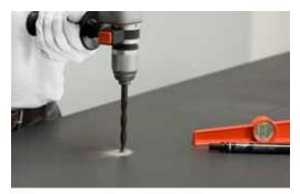
For holes having a max. diameter **8-10 mm**, use diamond or tungsten bits for glass or porcelain stoneware mounted on electric drills. Do not hammer-drill and start with a slow rotation speed. Do not press too much on the surface. It is recommended to cool the tool and the drilling point with water.
