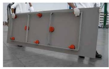
To aid handling of **1000x3000 mm** slabs, above all to handle a slab weakened by drills or openings and to aid the wall application, a suitable frame with suckers can be used. This frame is available upon request and is shown in the price list. Always check the perfect adhesion of the suckers on the slabs before handling it.
