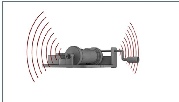
The melody only becomes louder when the vibration-distributing surface is enlarged. This happens as soon as the music box is placed on a table top. The vibrations from the music box are now transmitted to the table top. This part is called structure-borne sound.
