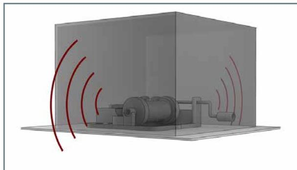
Elastic bedding with **Regupol®** and **Regufoam®**, adjusted to the machine in question, reduces the generation of the structure-borne sound.
