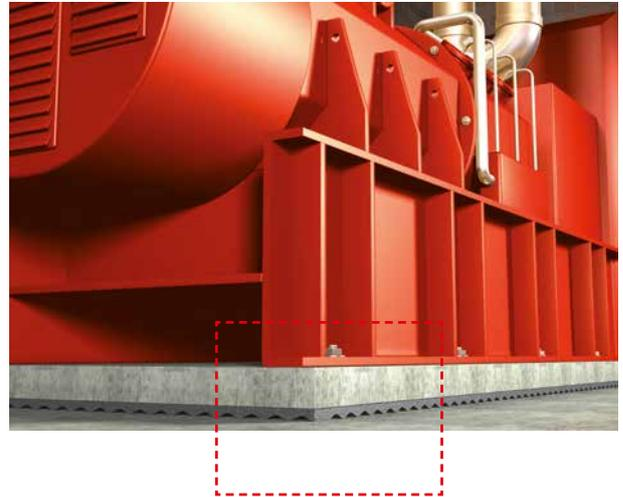
The isolation effect depends on the ratio between the natural frequency  $\omega_0$  and the interfering frequency  $\omega$ . The natural frequency should be below the lowest interfering frequency (low adjustment). The softer the elastomer and thus the lower the natural frequency, the better the isolation effect.
