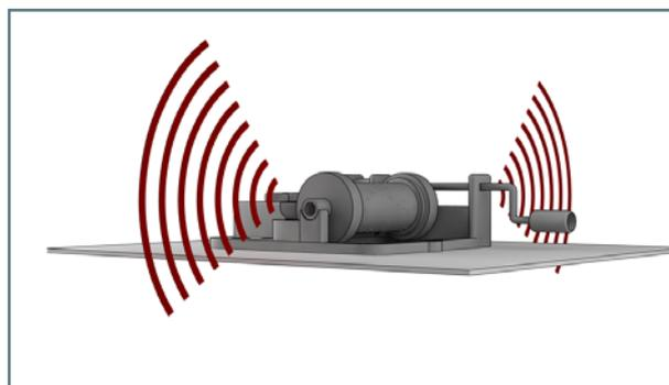
Imagine that this machine is placed inside your business, causing unacceptable noise. Often the first measure to be suggested is a sound protection hood, which usually, however, has no effect whatsoever.
